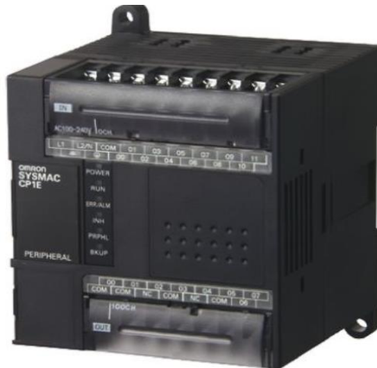
Fig.4: AVC- Embedded PLC
